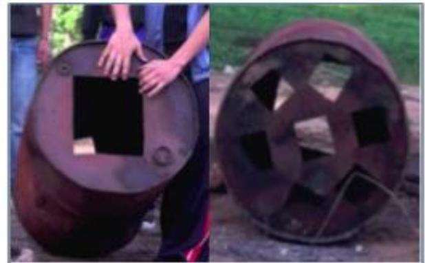
Figure 4: The finished drum with a square opening cut on top and seven holes on bottom
