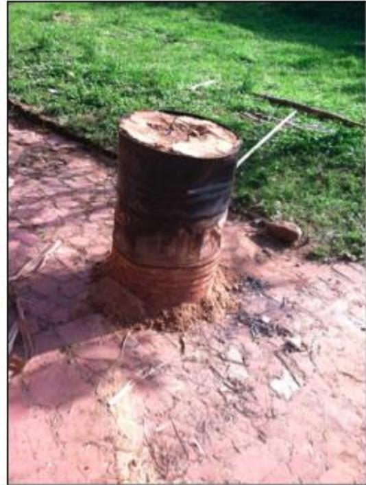
Figure 10: Sand was placed around the edges of the bottom and top of the drum to seal out oxygen
