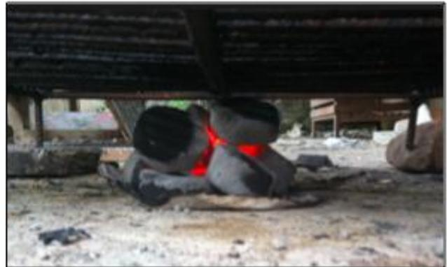
Figure 16: Briquettes made with cassava as an adhesive burning
