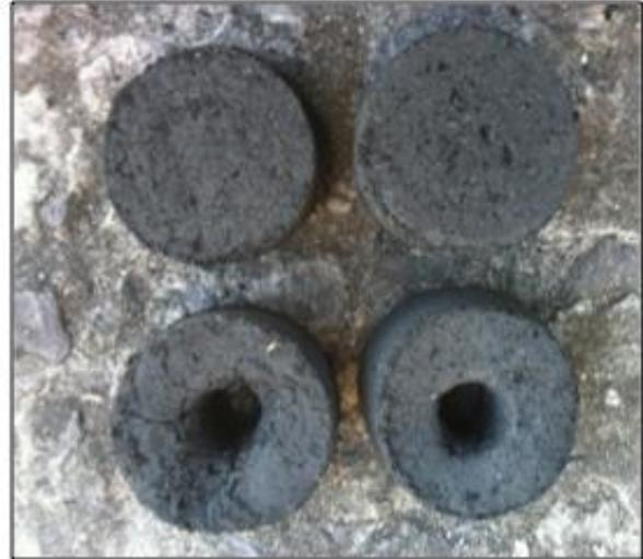
Figure 14: In the left column are briquettes made with banana as an adhesive and in the right column are briquettes made with cassava as an adhesive. In the first row are solid briquettes and in the second row are briquettes with holes in them
