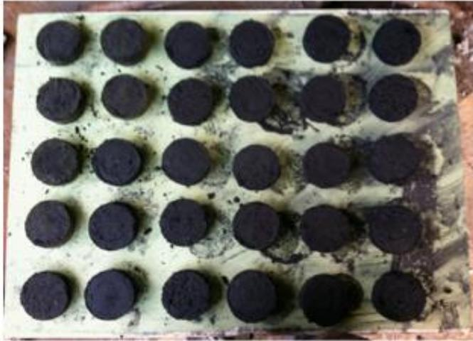
Figure 13: A tray of moist briquettes ready to dry in the sun. Charcoal is generally black in color, while ash is greyer; therefore, darker briquettes are desired
