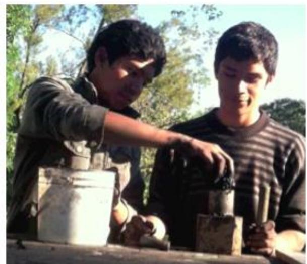
Figure 12: A lump of dough from the mix of water, cassava powder, and pulverized charcoal in the white bucket being placed in the press
