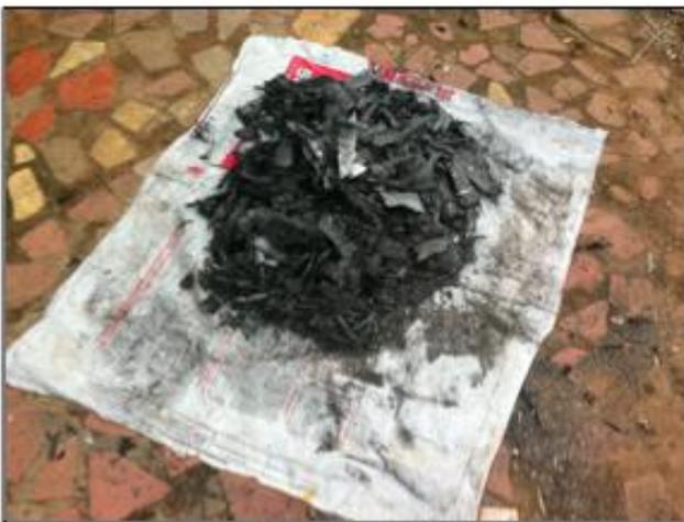
Figure 11: A charcoal yield from one burn. Most of the agricultural waste had successfully carbonized
